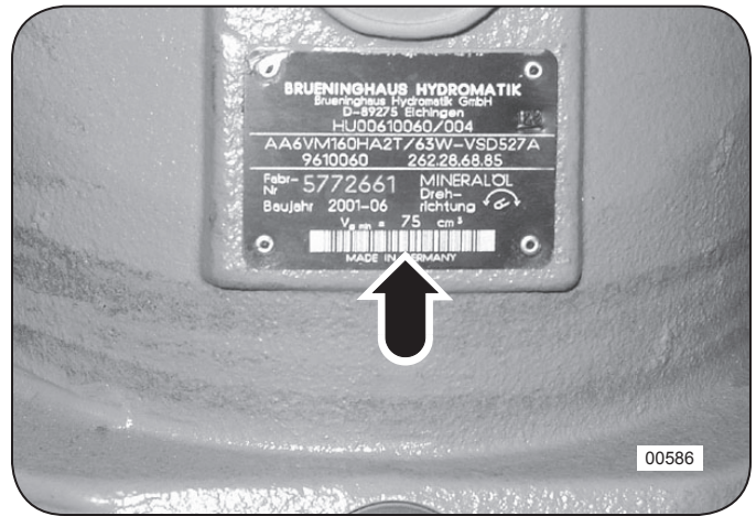
Figure 15: Motor S/N# Tag (Markings directly above the bar code identify this motor as a 70cc)
