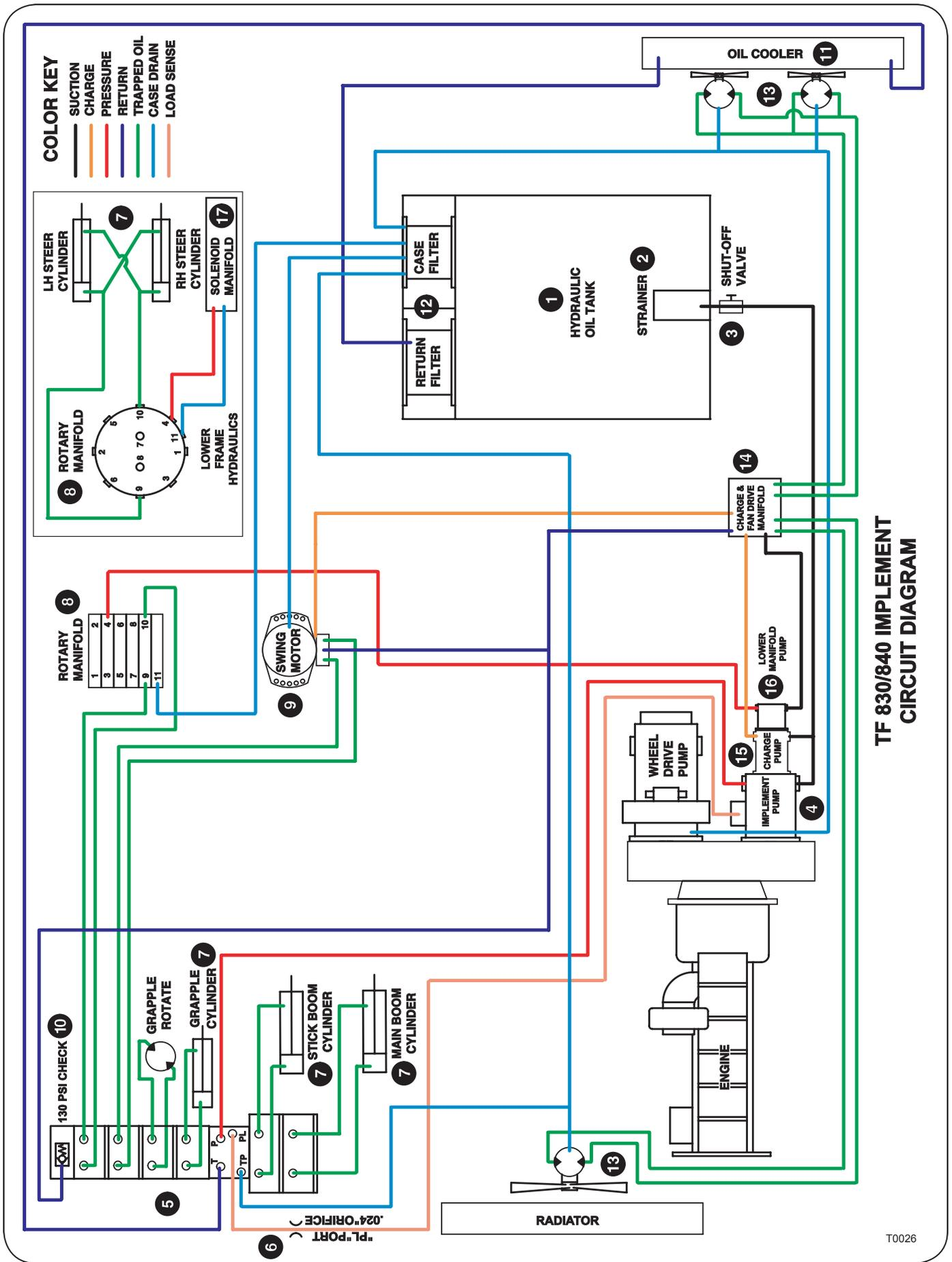
Figure 1: Simplified TF 830 Implement Circuit Diagram (Typical)
