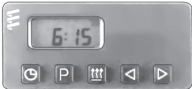
The 7 Day Timer has been designed to provide a simple means to control the operation of the heater system and to include the capability for diagnostics. This timer connects to the diagnostic circuit of the heater. The timer then displays any heater fault codes in three digit number form automatically. The timer allows for pre-selection of turn on time, up to 7 days in
