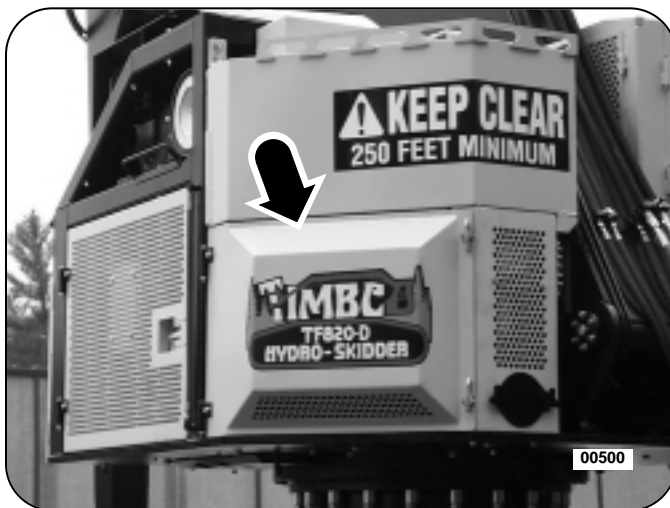
Figure 18: Swing-Out Pump Access Guard
