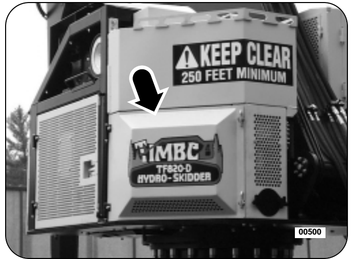
Figure 6: Swing-Out Pump Access Guard
