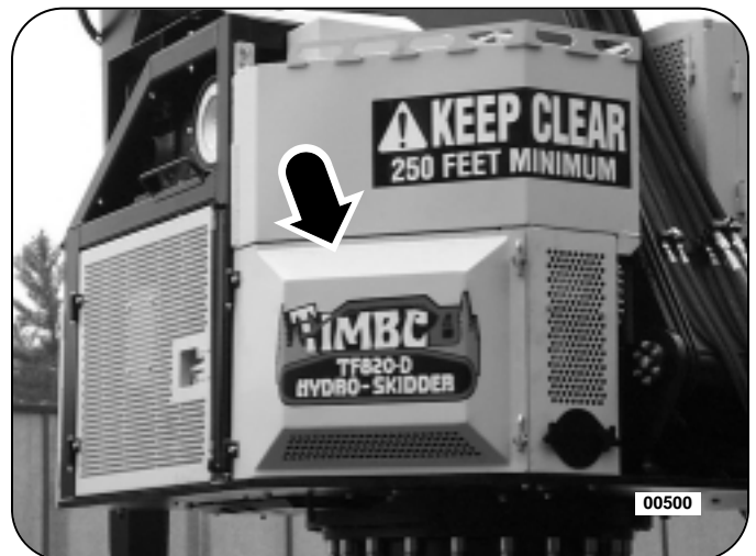
Figure 35: Swing-Out Pump Access Guard
