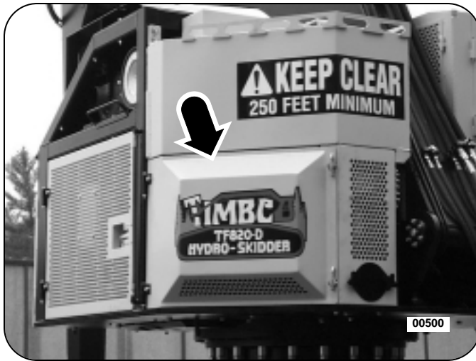
Figure 11: Swing-Out Pump Access Guard
