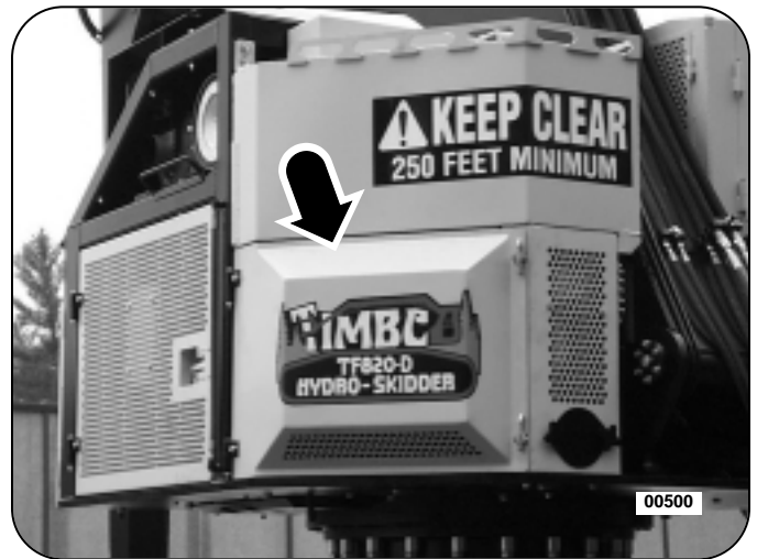
Figure 14: Swing-Out Pump Access Guard
