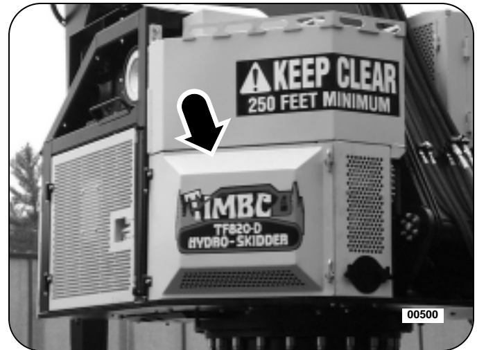
Figure 2: Swing-Out Pump Access Guard
