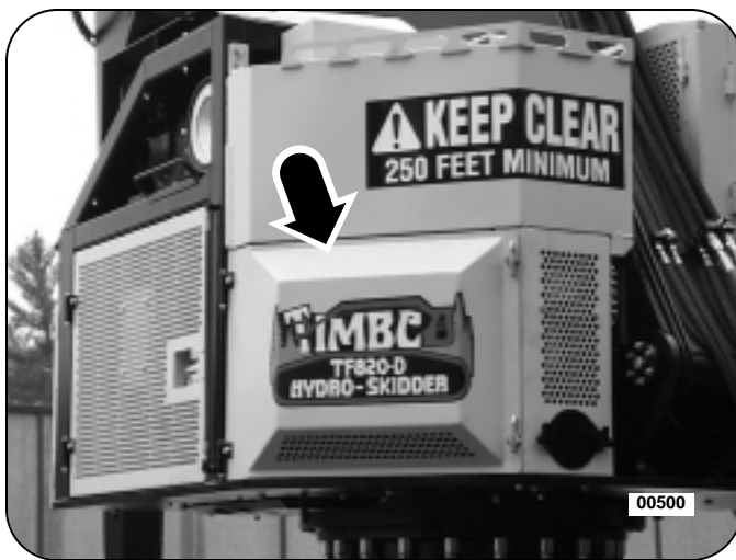
Figure 28: Swing-Out Pump Access Guard
