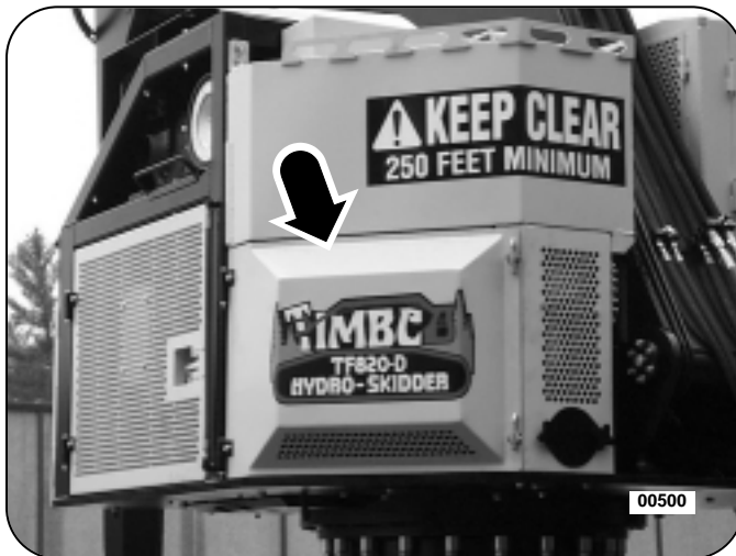
Figure 31: Swing-Out Pump Access Guard
