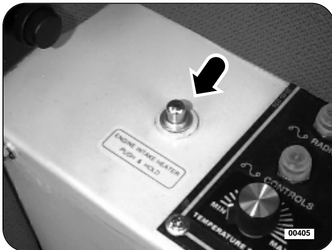
Figure 6: Caterpillar Engine Air Intake Pre-Heat
