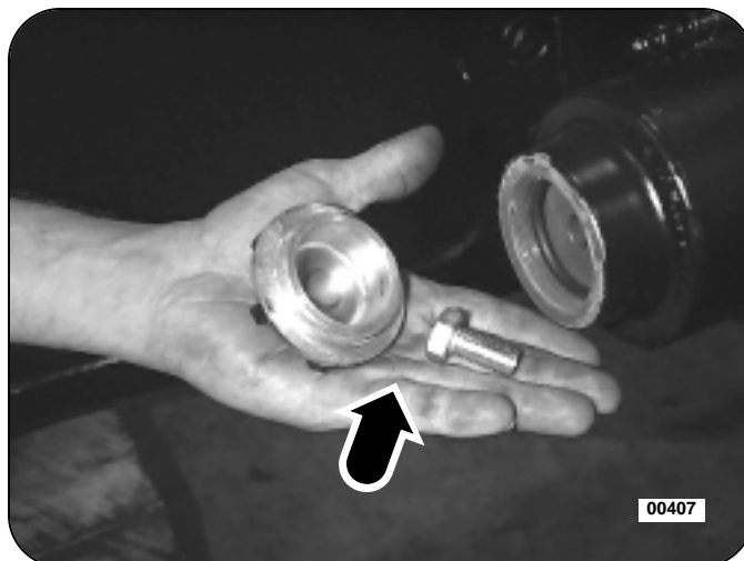
Figure 4: Parking Brake Manual Release Screws
