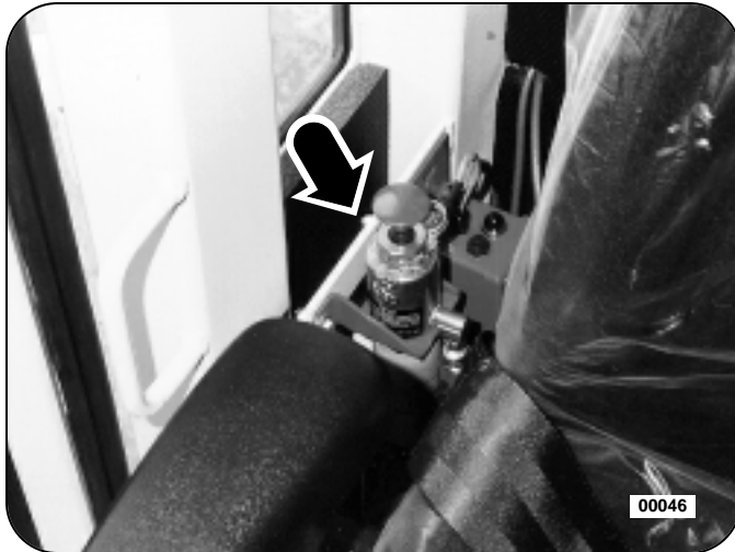
Figure 15: Optional Fire Suppression In-cab Manual Actuator And System Operation Test Box
