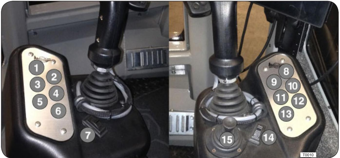
Figure 1: Machine Control Pods
