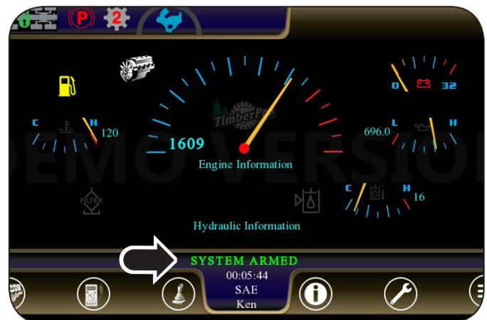
Figure 2: System Armed and Park Brake Light activate the charge oil heater. A message for the charge heater should now be displayed on the MD4 screen. Push down on the charge heater switch again to de-activate the charge heater system.
