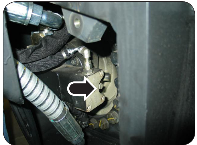
Figure 20: Drive Motor Begin Of Stroke Adjustment
