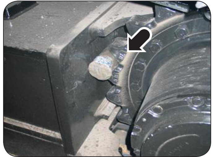
Figure 13: Lock Pin in Sprocket
