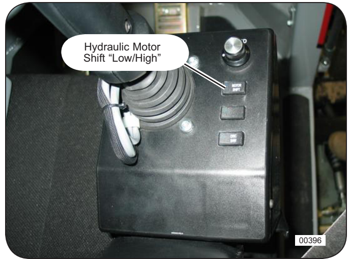
Figure 14: Hydraulic Motor Shift Control
