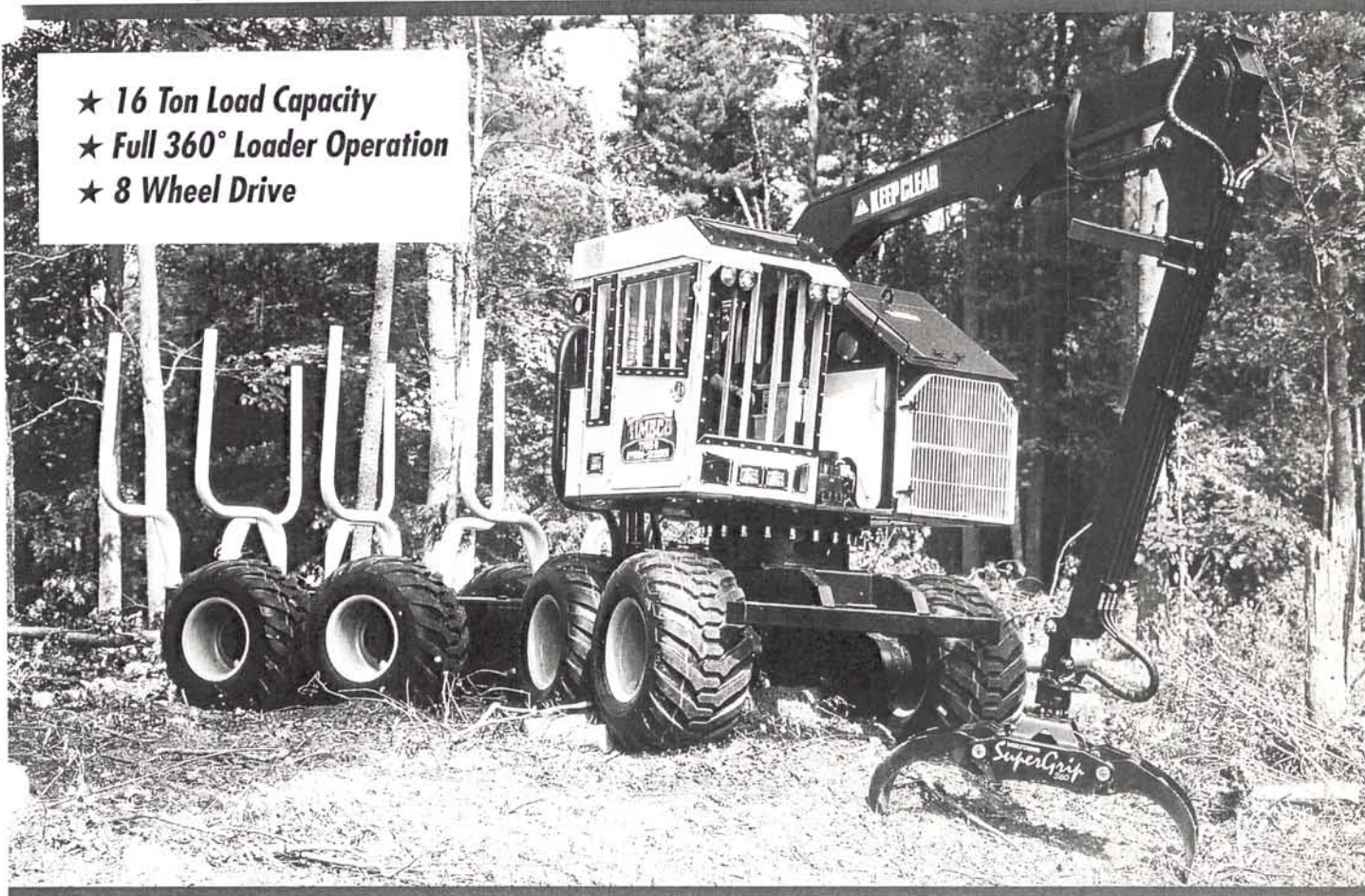
Timbco TF815 shown in Forwarder configuration.
