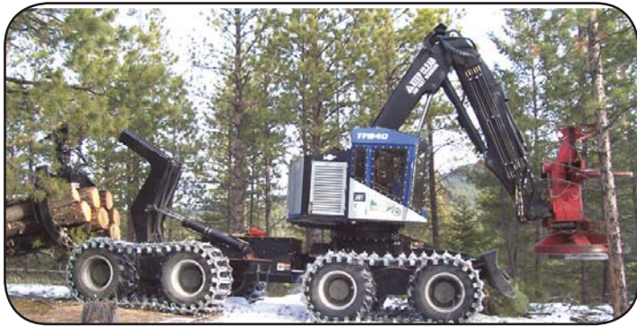
TimberPro TF 840 Shown with Optional Feller Buncher Booms, Arch Grapple, and Custom Quick Change adapter to allow removal of disc saw and installation of grapple to reduce weight when skidding.
