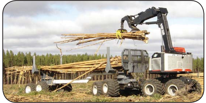
TimberPro TF 840 Forwarding eucalyptus in Australia. Shown with Optional Feller Buncher Booms, Live Heel, and Custom Trailer.
